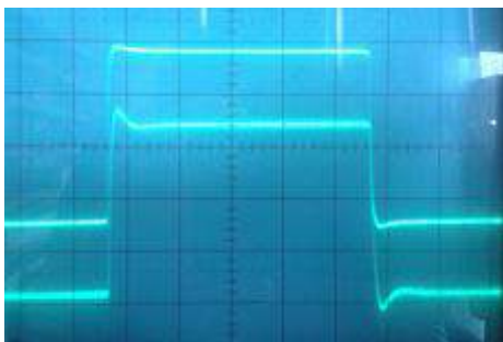
Pulse current signal response characteristic
